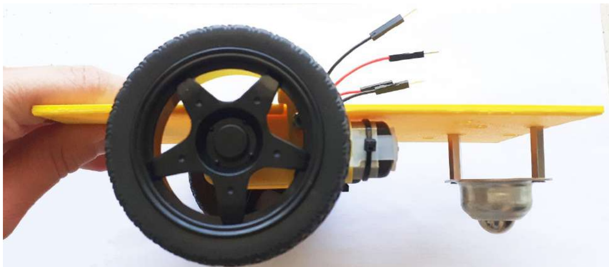
Figure 12: The DIY robotic car after placing all the components at the bottom side of the chassis
