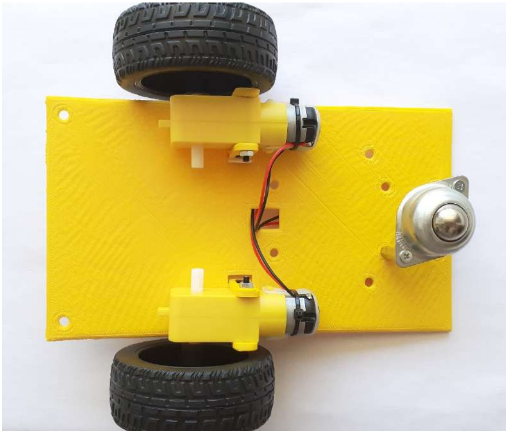
Figure 11: The DIY robotic car after placing the last part at the bottom side of the chassis
