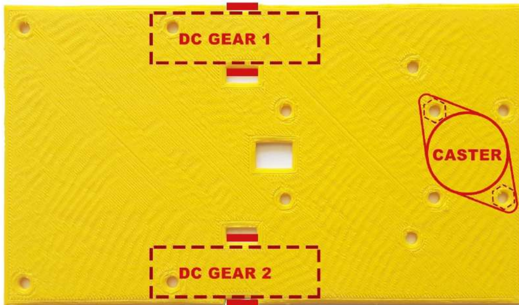
Figure 9: Diagram showing where the ball caster should be mounted
