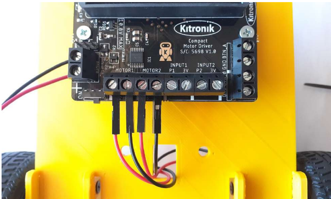
Figure 21: Connecting the two DC gear motors to the Compact motor driver
