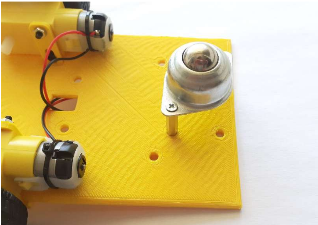
Figure 10: Mounting the ball caster on the chassis
